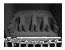
b) Position the two halves of the front ceramic (L/H & R/H) on the locating channel in the front ceramic, ensuring it is located onto the lip on the burner front ceramic support. (See fig. 4 below)
